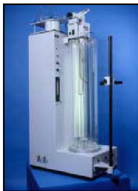
Figure 8.5 Equipment for Measuring Density of Samples of Plastic (Ametek, Lloyd Instruments Ltd)
