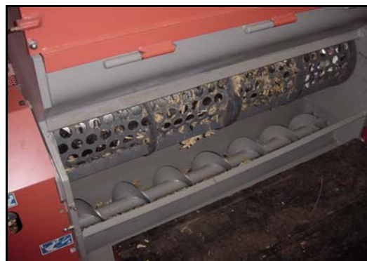
Figure 7.3 Shredder to reduce plastics to 15-50 mm pieces (Untha)
