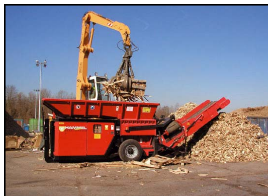
Figure 7.2 Large Aperture Shredder to pre-shred large items of plastics, shown here shredding timber
